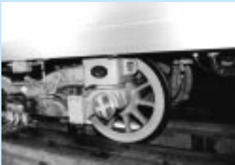
Wheel under Q/P Measurement
